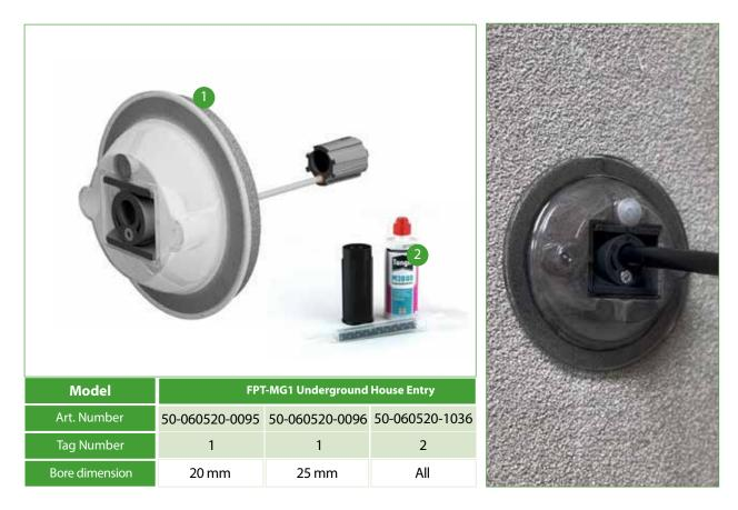
1: FPT-MG1 Underground House Entry / tiltable Below Ground House Entry. For out-door installation. Gas and watertight up to 1 bar. Horizontal and incline istallation is possible due to the smart hinge design. MG-1 is usable in all wall thicknesses.
