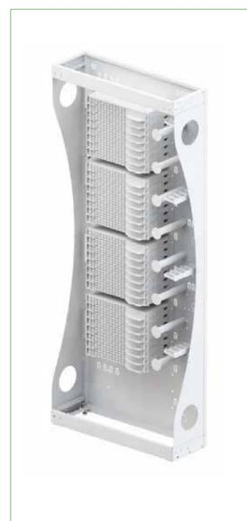
ModelPatchmodul Type 1Art.Nr.43-0903.01Dimensions WxHxD900x2174x300 mmCabinet materialpainted SteelWeight Racksystem51,48 kgWeight Set172.08 kgStandardsEIA/IEC/DINColourlight grey
